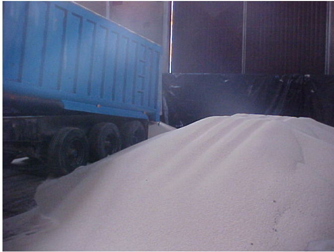
Bulk storage of ammonium nitrate
