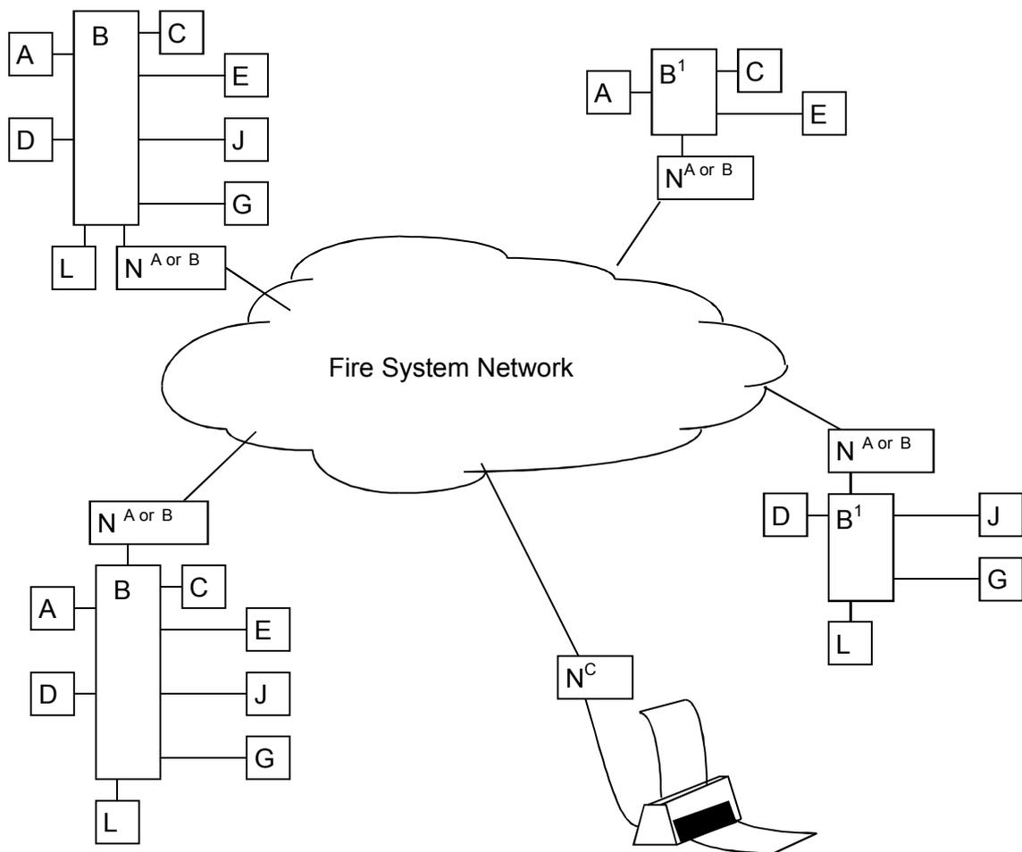
Figure B1: Example of a Fire System Network in relation to Control and Indicating Equipment
