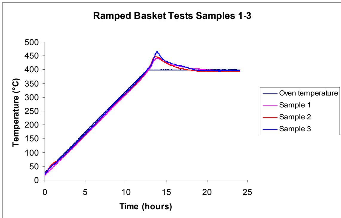
The figure above shows a test trace for a material exhibiting self-heating behaviour.
