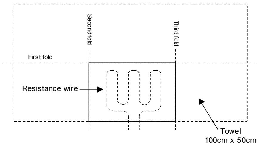
**Figure I.1 - Arrangement of the cotton towel and ignition source**
