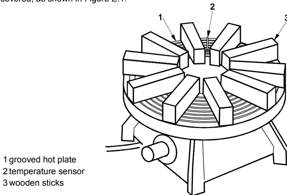
**Figure E.1 — Arrangement of the sticks on the hotplate**
