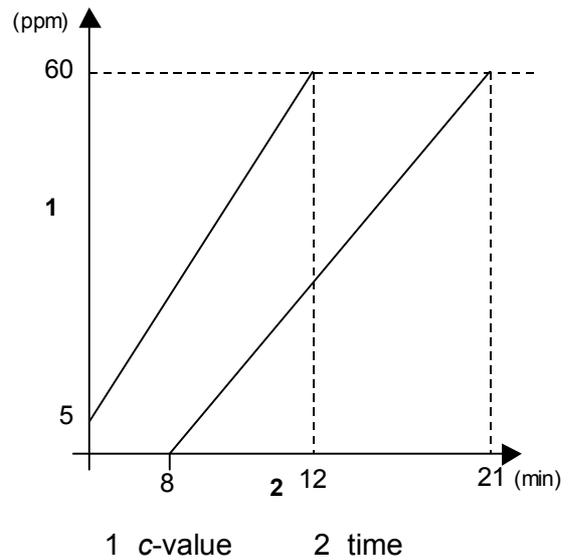
**Figure I.3 — Limits for  $c$  against time, Deep-seated smouldering cotton fire**
