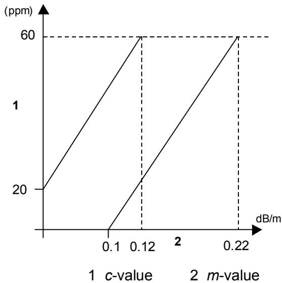
**Figure I.2 — Limits for  $c$  against  $m$ , Deep-seated smouldering cotton fire**
