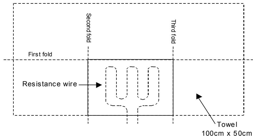
**Figure G.1 - Arrangement of the cotton towel and ignition source**
