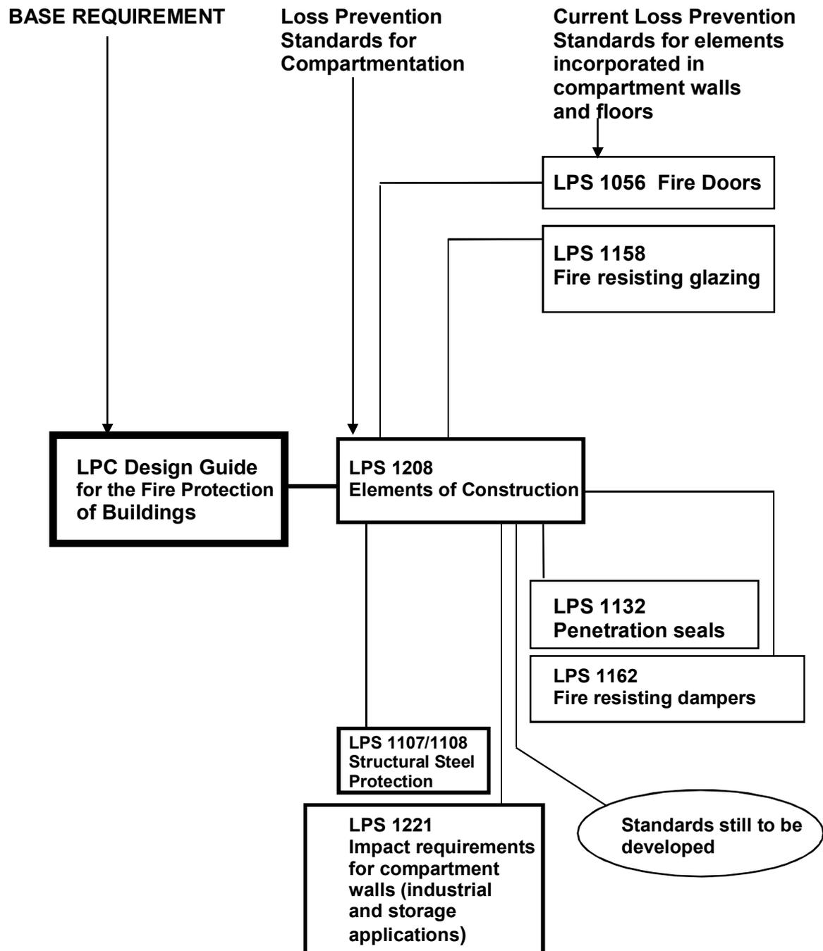
**NOTE: THIS DIAGRAM INTENDS TO ILLUSTRATE THE COMBINED ROLE OF PASSIVE FIRE PROTECTION SYSTEMS TO MAINTAIN COMPARTMENTATION**
