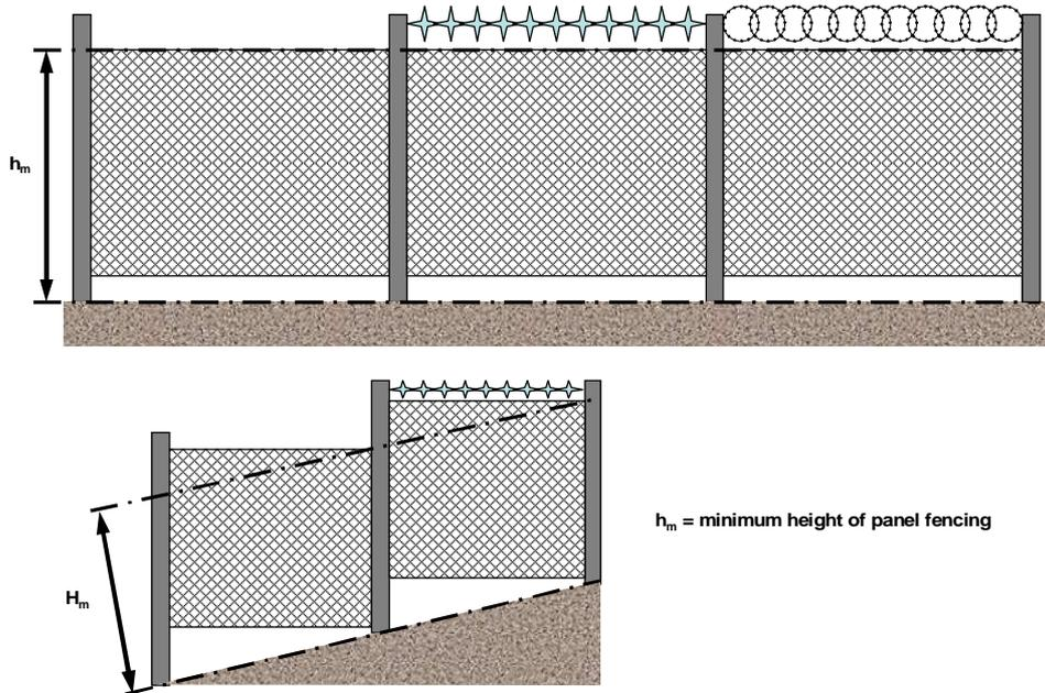
**Figure 3** Minimum height of free-standing barriers - palisade fencing
